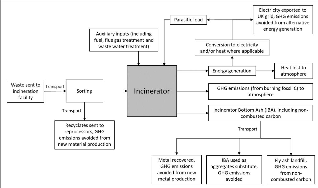
**Figure 7. System boundaries for sending one tonne of waste to a gasifier**
