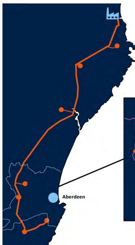
Aberdeen Vision, which is near completion, has routed and designed the pipeline connecting hydrogen production at St Fergus terminal with the required infrastructure to enable conversion to Aberdeenshire including the city of Aberdeen. This project has progressed to pre-FEED level.<sup>6</sup>
