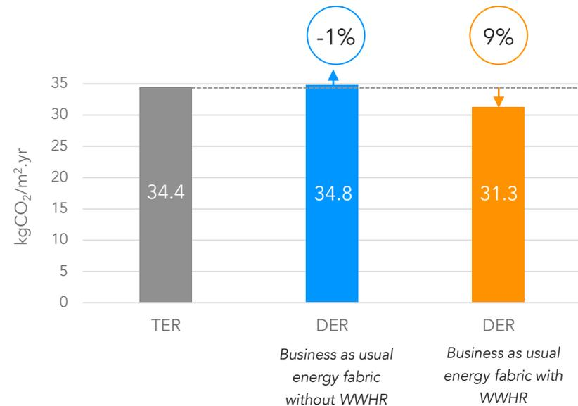
Figure 6.5 - The chart above shows the impact of WWHR on the GLA ‘Be Lean’ case in a mid-rise apartment building. A significantly greater reduction in CO<sub>2</sub> emissions is achieved when WWHR is included in the proposed building specification.
