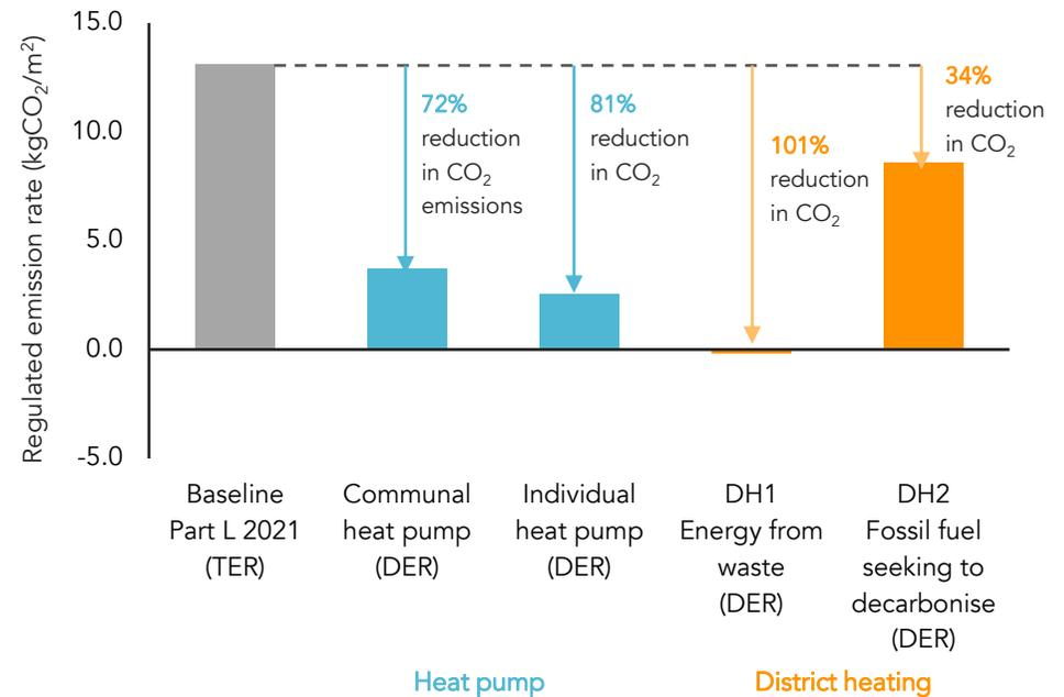
Figure 6.9 - Analysis of district heating and comparison with heat pump scenario
