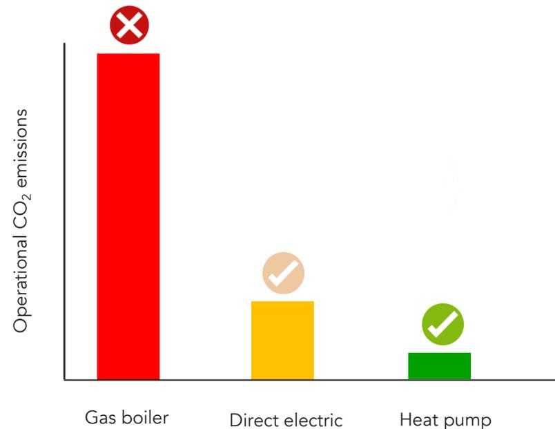
Figure 11.11 - The choice of heating system will affect operational CO<sub>2</sub> emissions over a long time. Electric forms of heating (direct electric and heat pumps) will emit a fraction of a gas boiler carbon emissions (see above the average over 2022-2050)
